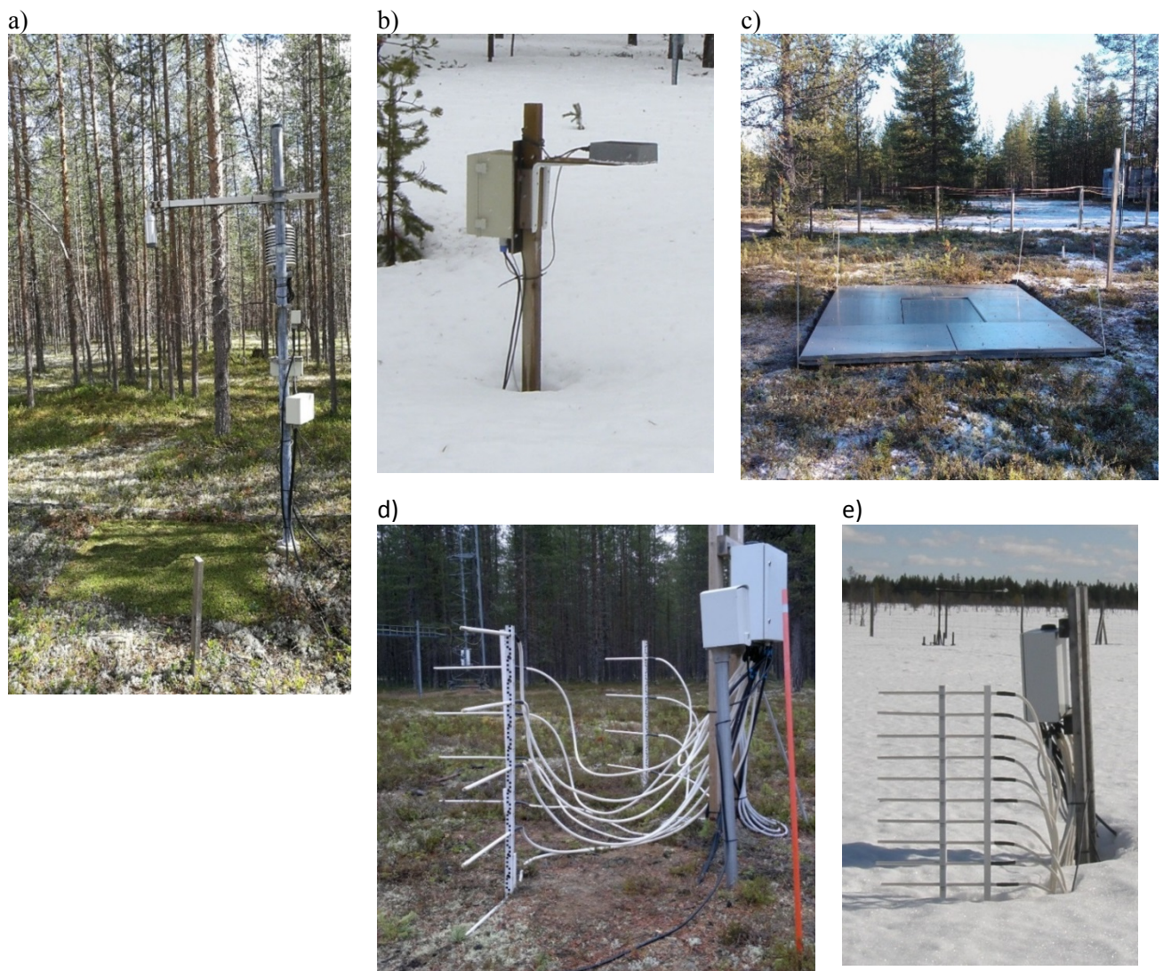
Fig. 2. a) A weather station with an SR50 sensor in sparse pine forest at the IOA, b) GWI at in forest clearing IOA and c) SSG1000 at IOA. Snow temperature profiles d) at IOA (installation every 30 cm in three poles) and e) at bog site (installation every 10 cm).
