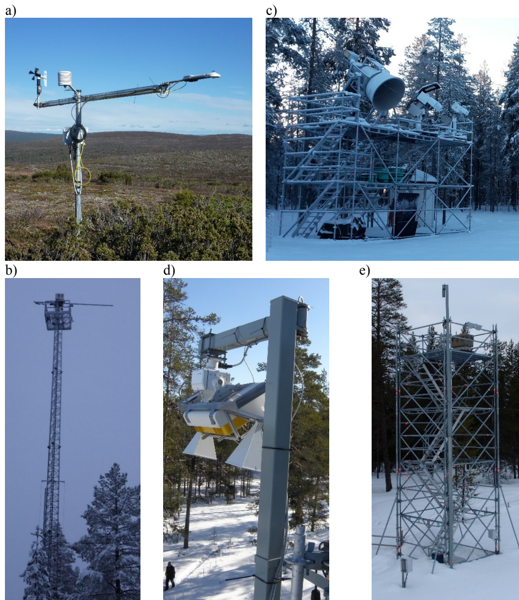
Fig. 3. a) CNR4 albedometer at Saariselkä. Thermometer and wind sensor are installed on the same bar, b) optical spectroradiometer FieldSpec Pro JR installed on 30 m mast, c) ESA ELBARA-II, SodRad1 and SodRad2 radiometers on 4 m tower, and d) ESA SnowScat scatterometer and e) SodScat scatterometer on 8 m tower.
