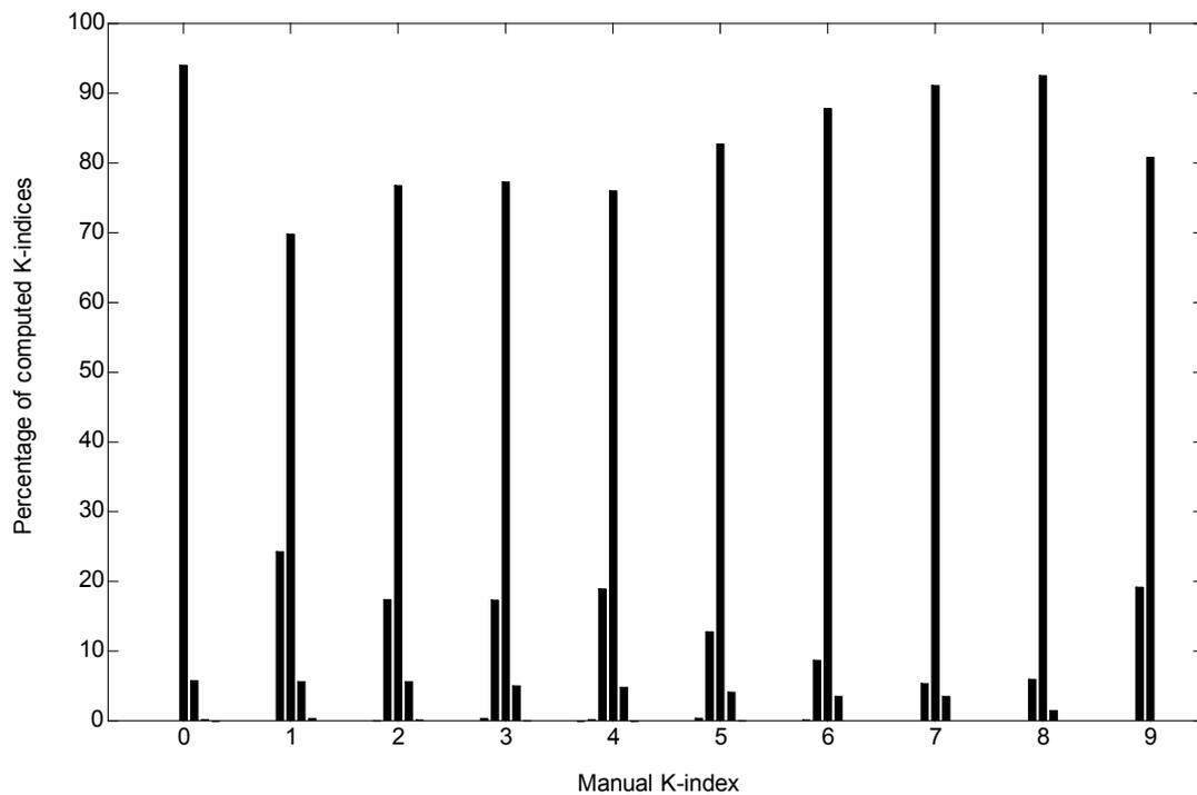
Fig. 2. Comparison between manual (MK) and computer produced (AK)  $K$ -indices at the Sodankylä observatory for the time frame Jan 1996 – May 2010. The bars at  $MK = 0, 1, \dots, 9$  give the percentage of AK-values that are equal to MK. The bar on its left/right side gives the percentage that the AK-value is one  $K$ -unit smaller/greater than MK.
