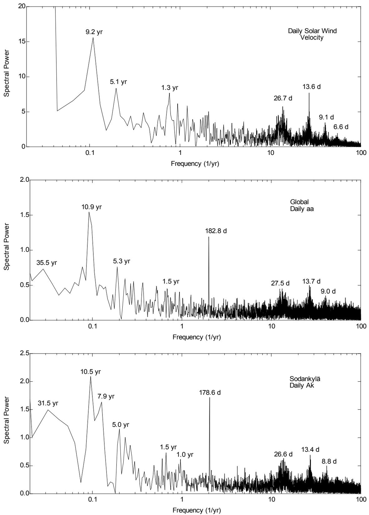
Fig. 3. Power spectrum of daily solar wind velocity (upper panel), global *aa*-index (mid-panel), and Sodankylä *Ak*-numbers (lower panel). Prominent spectral lines are attached by the period of the wave.
