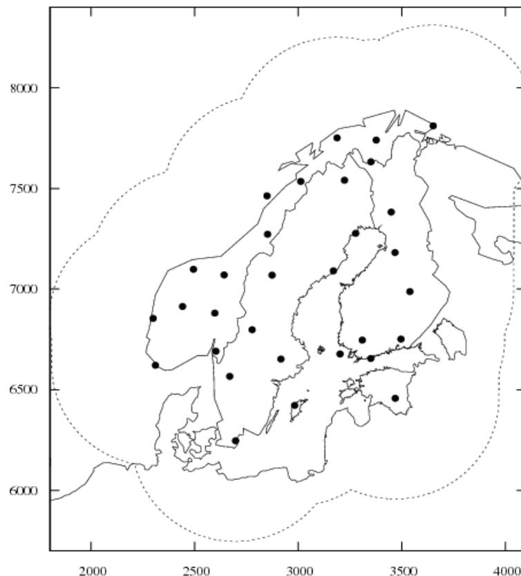
Fig. 2. NORDLIS lightning location system. Black circles are sensor locations, and the dashed line indicates the coverage area. X- and y-axis values are kilometres to the East and North, respectively.
