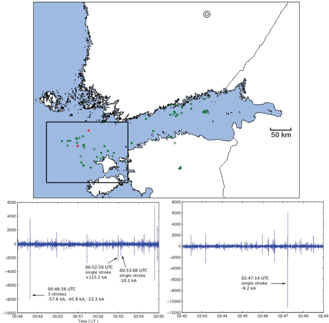
Fig. 4. Upper: CG locations from Oct 9 2009. Plus-signs and filled circles indicate positive and negative CGs, respectively. Red coloured locations are the suspected parent flashes of the TLEs. The double circles indicate the camera position. Below: Pulsation magnetometer observations recorded at Sodankylä (67.42°N, 26.39°E), approximately 950 km from the thunderstorm. Some of the located flashes are visible in the waveforms.
