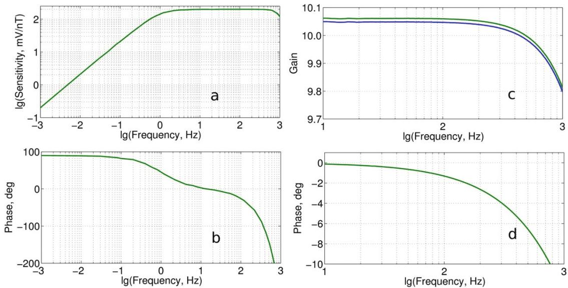
Fig. 4. Transfer functions of the two magnetic (H) channels (= difference between input and output signal as a function of frequency) and electric (E) channels. (a) Sensitivity of H channels, (b) phase of the transfer functions of H channels, (c) gain factor of E channels and (d) phase of the transfer functions of E channels.
