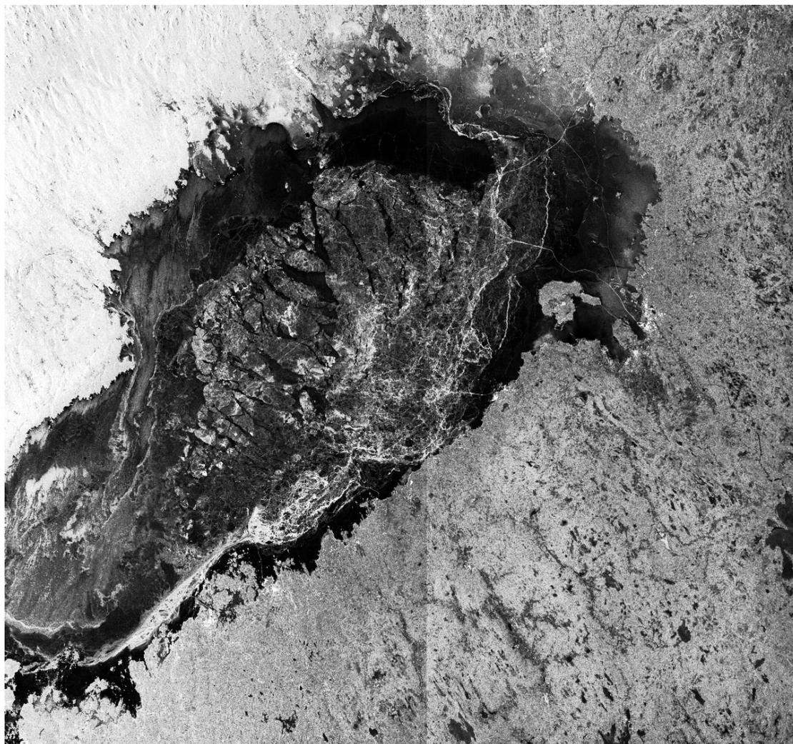
Fig. 1. The ice cover of the Bay of Bothnia on 17 March 1997 during the ZIP-97 experiment, in a section of Radarsat SAR image (Sandven et al., 1999). © Canadian Space Agency.
