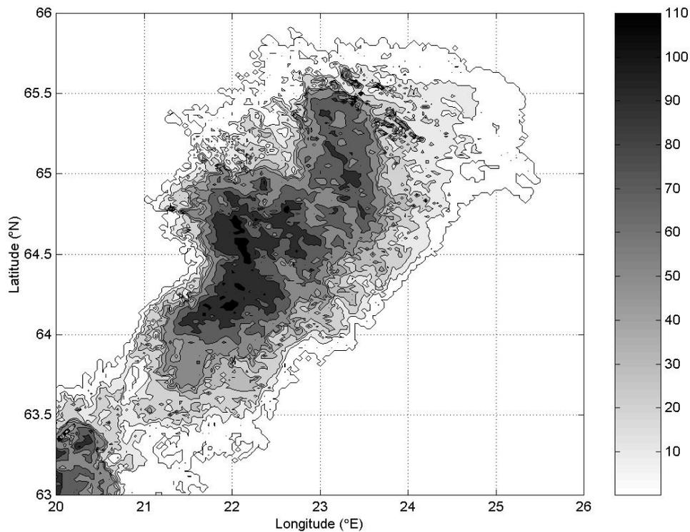
Fig. 2. Bathymetric chart of the Bay of Bothnia.
