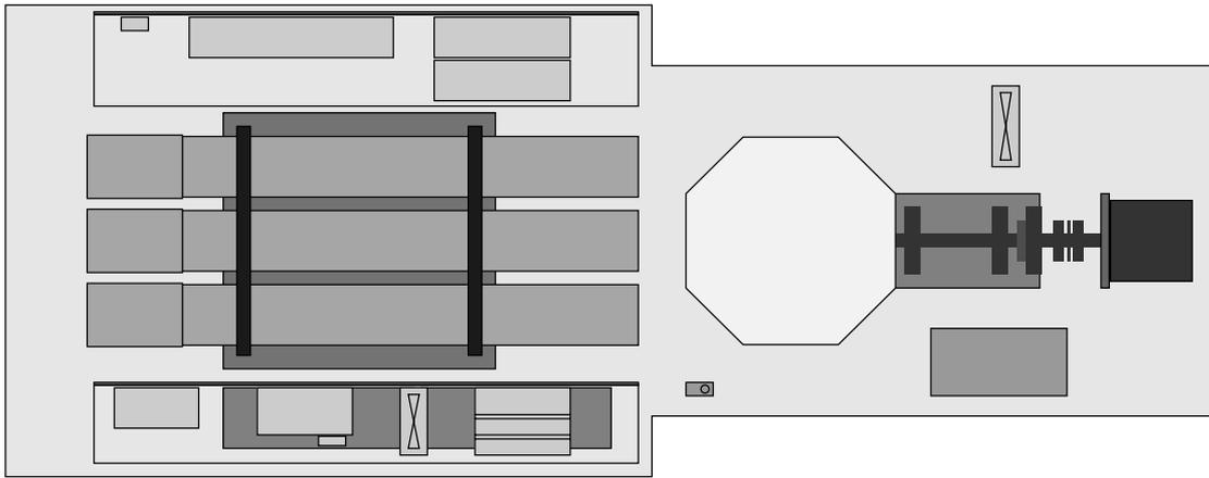
Fig. 3. A schematic top view of an auroral photometer. On the left center there is a block of photometer tubes, above it there is a high voltage block. On the lower left there are the main switch, heating and other power supplies in its own module. On the right side there is the scanning module with an octagonal mirror, stepping motor with its driver and absolute angle encoder.
