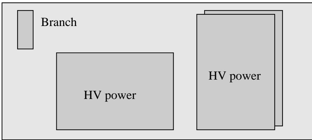
Fig. 5. The high voltage block consists of three Bertan high voltage power supplies, one in the middle and two on the right side.
