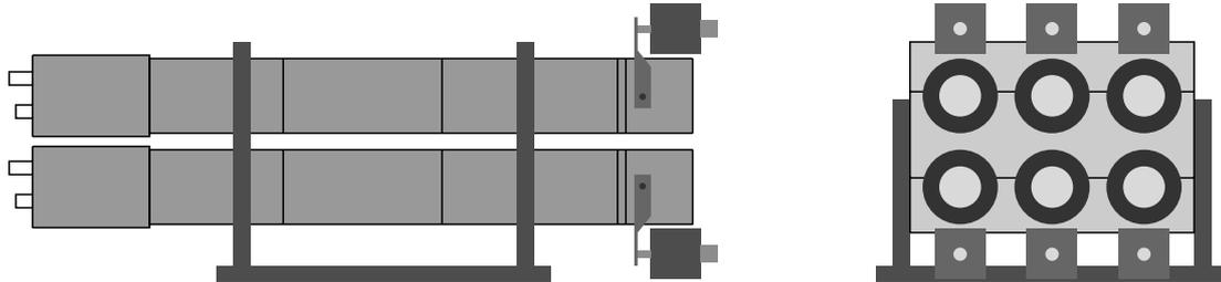
Fig. 8. All the photometer tubes are mounted in a tight block. Here the block is seen from side (left) and front (right).
