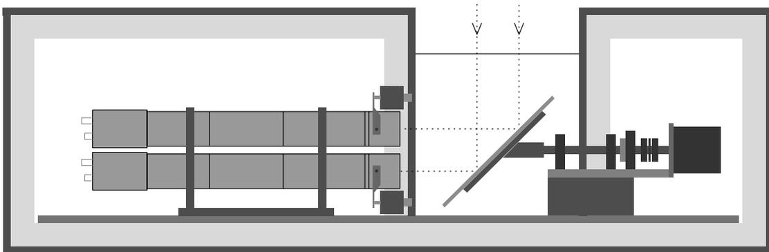
Fig. 2. A schematic side view of an auroral photometer box. On the left there is a block of photometer tubes. The scanning module is on the right. The light enters to the box via a cylindrical acrylic window and reflects from the first surface mirror to the photometer tubes. The light beams are marked with dashed lines.
