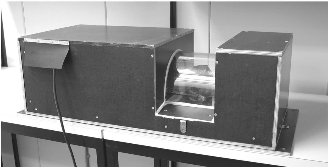
Fig. 1. On the top: The scanning auroral photometer in the laboratory. Bottom: The same photometer mounted in its wooden box ready to operate in outdoor conditions.
