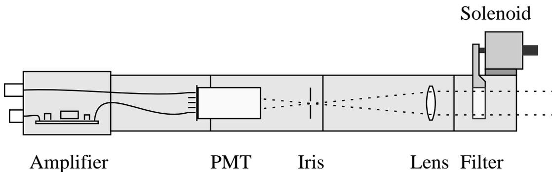
Fig. 4. A photometer tube consists from right to left: a filter and the tilting solenoid, lens, iris, photomultiplier tube (PMT) and amplifier.
