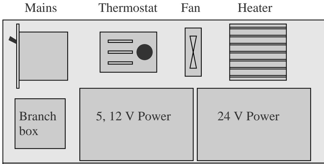
Fig. 6. The other power supply block contains the mains, heating system and the low voltage power supplies.
