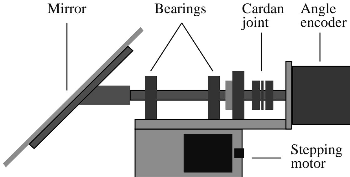
Fig. 7. In the scanning system of the photometer a first surface mirror is installed at an angle of  $45^\circ$  to the scanning axis. The stepper motor below is turning the axis and at the end of the axis there is an absolute angle encoder.
