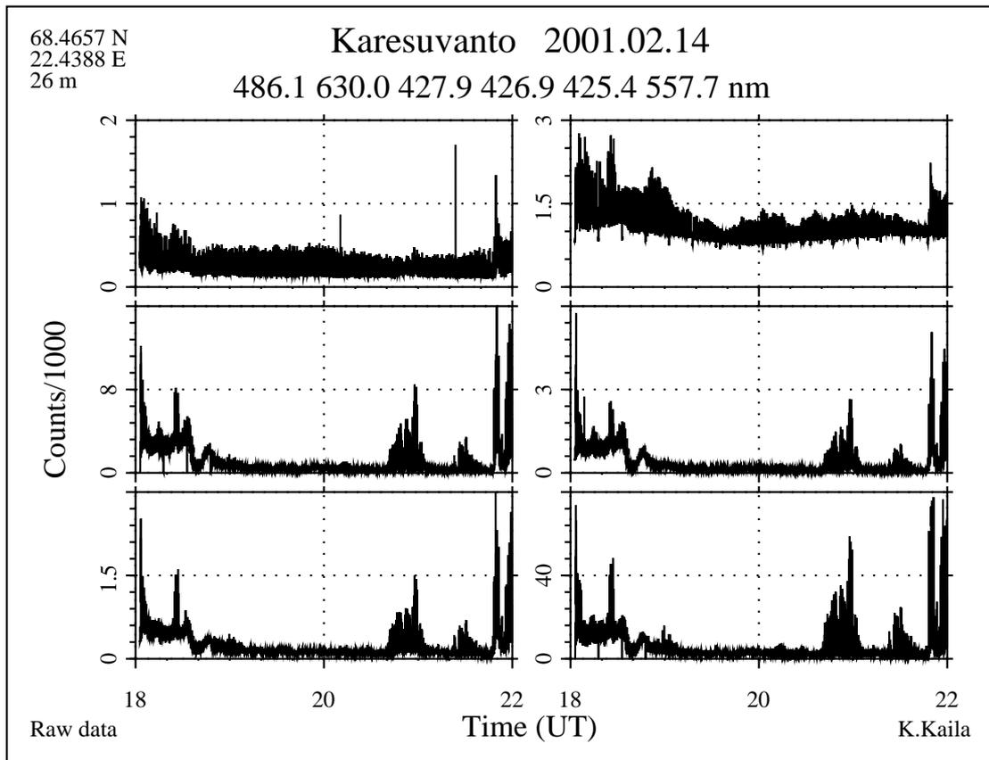
Fig. 9. An example of the photometer recording from Karesuvanto on 14.02.2001 at 18:00-22:00 UT. The station name, date and wavelengths of following panels are shown at the top. The position obtained from GPS is seen in the upper left corner.
