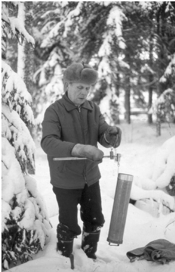
Fig. 2. Mr. Oiva Urjankangas is weighing a snow sample with a Korhonen-Melander device in the 1970s (photograph by Esko Kuusisto).
