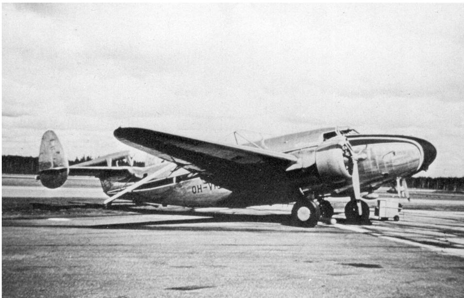
Fig. 9. The Lockheed Lodestar plane and the airborne EM system of GSF used from 1953. (*Ketola, 1986*; courtesy: M. Ketola.)
