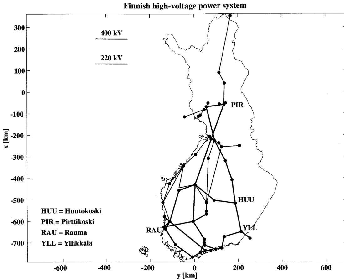
Fig. 19. The present-day configuration of the Finnish 220 and 400 kV power transmission system (*Pirjola et al., 2000*).
