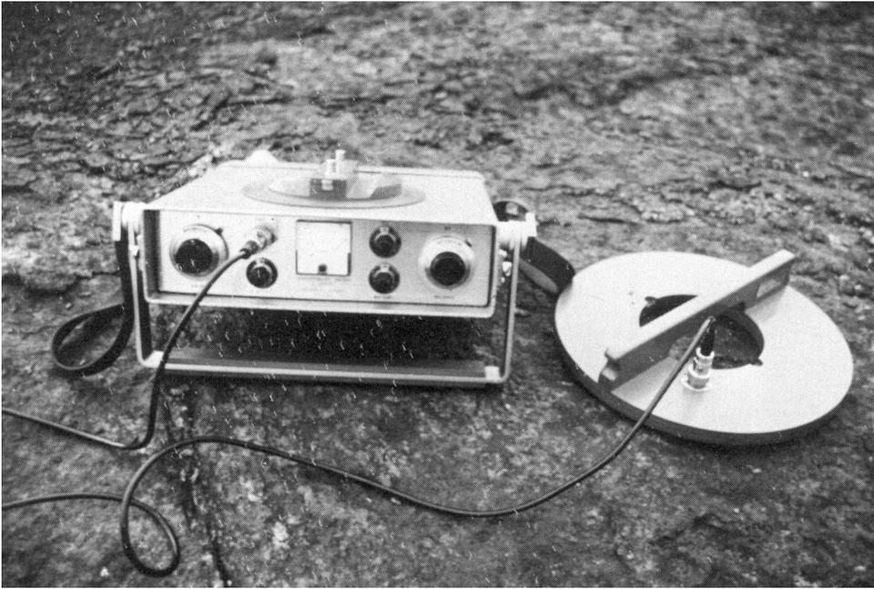
Fig. 11. Field susceptibility meter designed by GSF in the 1970's. (Ketola, 1986; courtesy: M. Ketola.)
