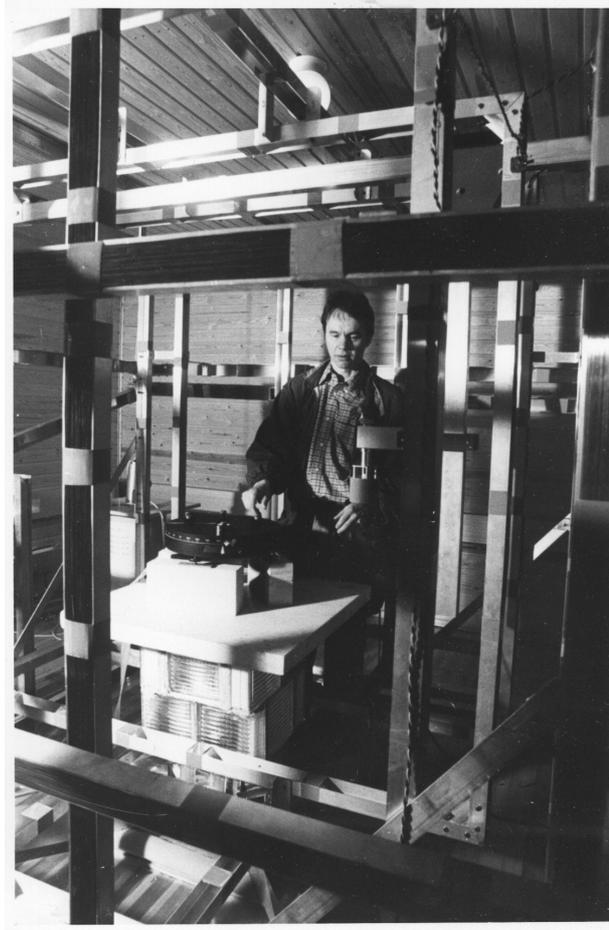
Fig. 5. Kari Pajunpää inside the calibration coil at magnetic test laboratory of the Nurmijärvi Geophysical Observatory (photo: Nanni Akkola).
