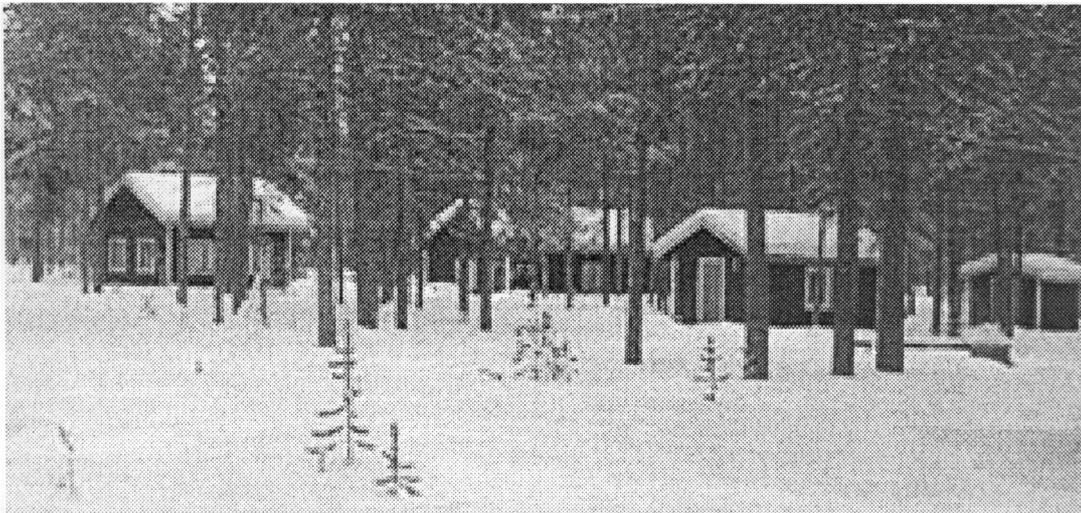
Fig. 3. Magnetic observatory registrations require (magnetically) quiet and homogeneous surroundings. The huts are built without a single piece of metal. (SGO, photo: Jyrki Manninen.)
