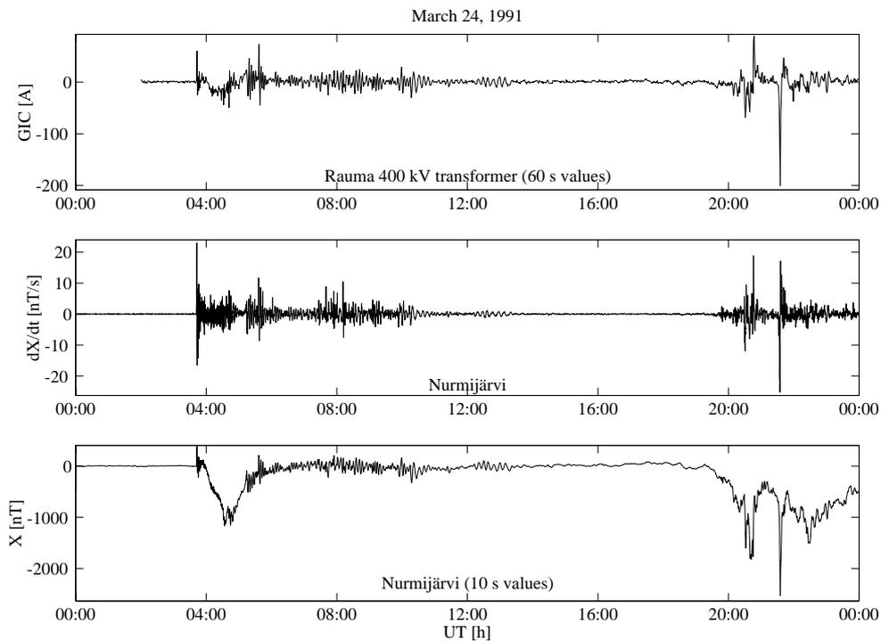
Fig. 20. GIC (positive into the Earth) in the earthing lead of the Rauma 400 kV transformer on March 24, 1991 (uppermost panel) and the simultaneous north component of the geomagnetic field (lowermost panel) and its time derivative (middle panel) at the Nurmijärvi Geophysical Observatory. (Pirjola *et al.*, 2000).
