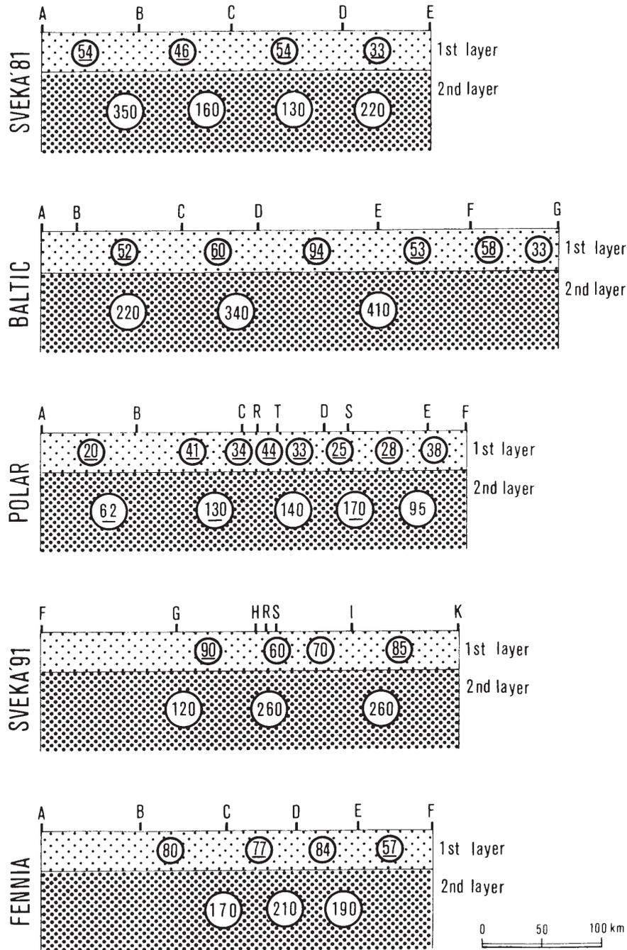
Fig. 8. Uppermost crustal structure along the deep seismic sounding profiles: SVEKA'81, BALTIC, POLAR, SVEKA'91 and FENNIA from Q<sub>R</sub> values of R-waves. Underlined values are average Q<sub>R</sub> factors obtained from neighboring shot points (as an example the value Q<sub>R</sub>=54 for profile SVEKA is an average from Q<sub>R</sub>=46 for SP A and Q<sub>R</sub>=62 for SP B); the 1st layer is an uppermost basement, thickness of about 1 km and the 2nd layer reaches a depth of about 4 km.
