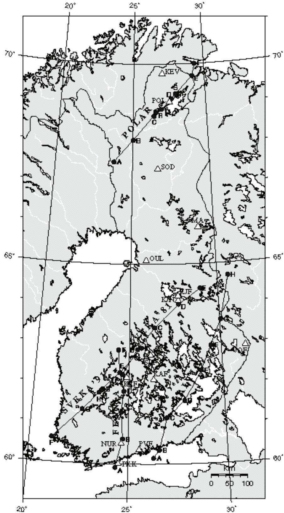
Fig. 1. Location of the deep seismic sounding profiles in Finland. Dots are shot points and triangles are permanent seismograph stations (with the exception of station POL), records of which were used in the analysis of amplitude - charge size dependencies.
