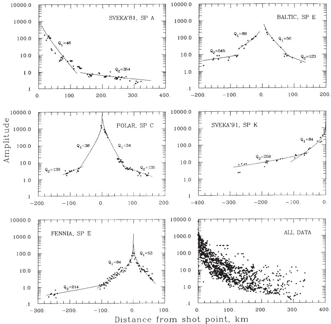
Fig. 7. Examples of observed amplitudes of R-waves for the SVEKA'81 (SP A), BALTIC (SP E), POLAR (SP C), SVEKA'91 (SP K), FENNIA (SP E) profiles and all the data.  $Q_1$  and  $Q_2$  values of quality factors according to formula (2).
