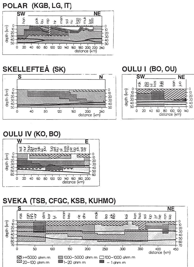
Fig. 5 Two-dimensional models of the POLAR, SKELLEFTEÅ, OULU I, OULU IV and SVEKA profiles. The resistivity scales of all models are the same and is shown in detail below the SVEKA model. The profiles have no vertical exaggeration. The thick black lines indicate the boundary between the upper and lower crust and the Moho boundary. Figure is from *Korja and Hjelt (1993)* where references for original studies are given.
