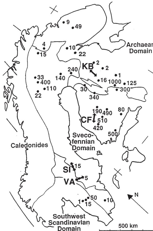
Fig. 8. Lateral variations in lower crustal conductivity. Solid arrows show the azimuth of the anisotropy (the most conductive direction) in those regions where magnetotelluric response functions representing deep crustal conductivity exhibit anisotropic features. VA=south-central Sweden; S=Siljan; CF=Central Finland Granitoid Complex and KB=Archaean Kuhmo block in eastern Finland. Figure is from Korja and Hjelt (1996).
