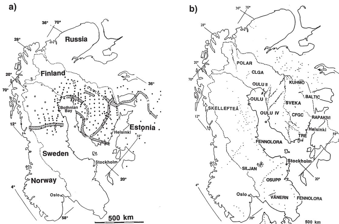
Fig. 4. Deep geoelectromagnetic studies in the Fennoscandian Shield. (a) Magnetometer sites and conductivity anomalies revealed by MV data. Central and southern Sweden have been covered by magnetometer arrays but the data have not been analysed yet. Ruled line: conductivity anomaly; dashed ruled line: conductivity boundary. (b) Magnetotelluric sites in the Fennoscandian Shield and the names of some profiles. Figure is from *Korja and Hjelt* (1993).
