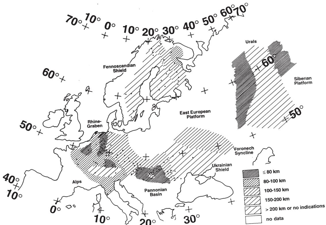
Fig. 2. A schematic map of the depths to the top of the electrical conductors coinciding approximately with the seismically defined lithosphere-asthenosphere boundary (LAB) in Europe (i.e. basically the first conducting layer in the upper mantle beneath the Moho which seems to coincide with the LAB although the electrical LAB is slightly deeper than the seismic LAB). Figure is from *Hjelt and Korja (1993)*.
