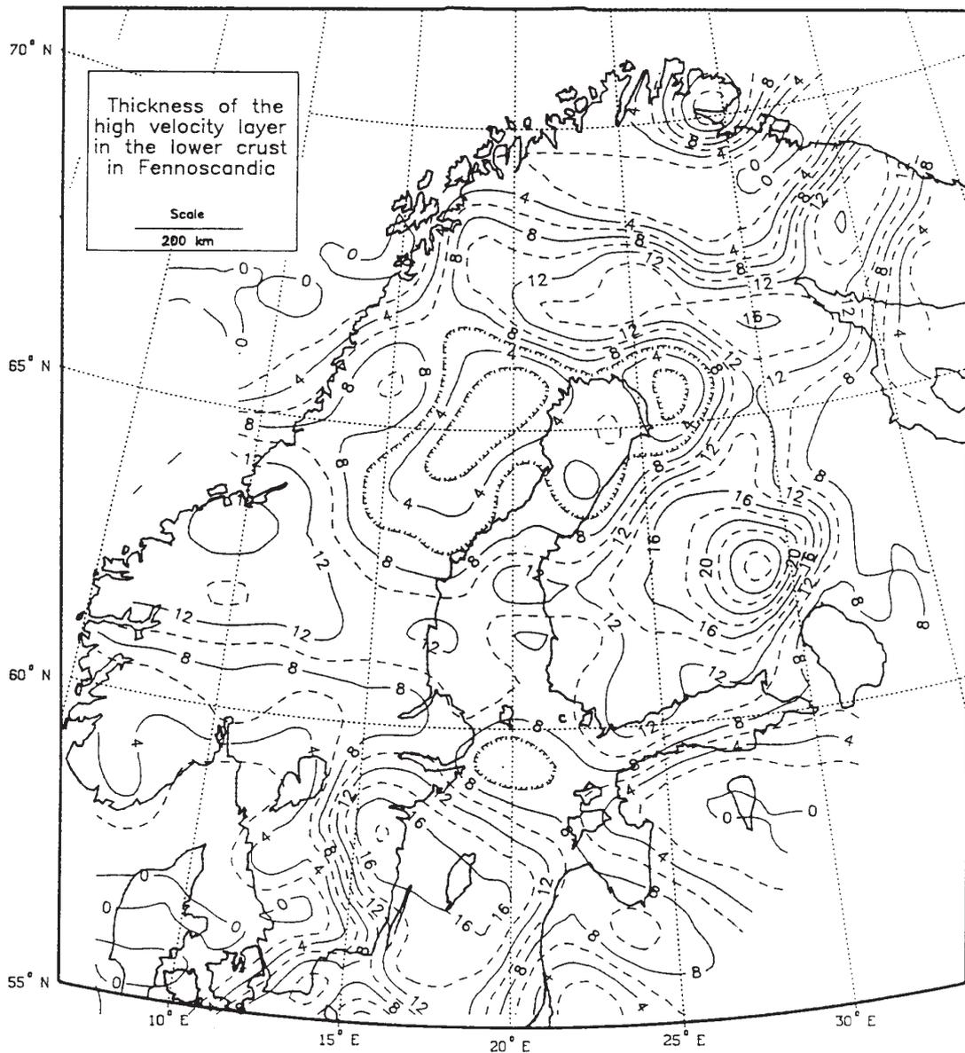
Fig. 5. Thickness (km) of the lowermost high-velocity crustal layer in Fennoscandia (Adopted from Korja et al., 1993).
