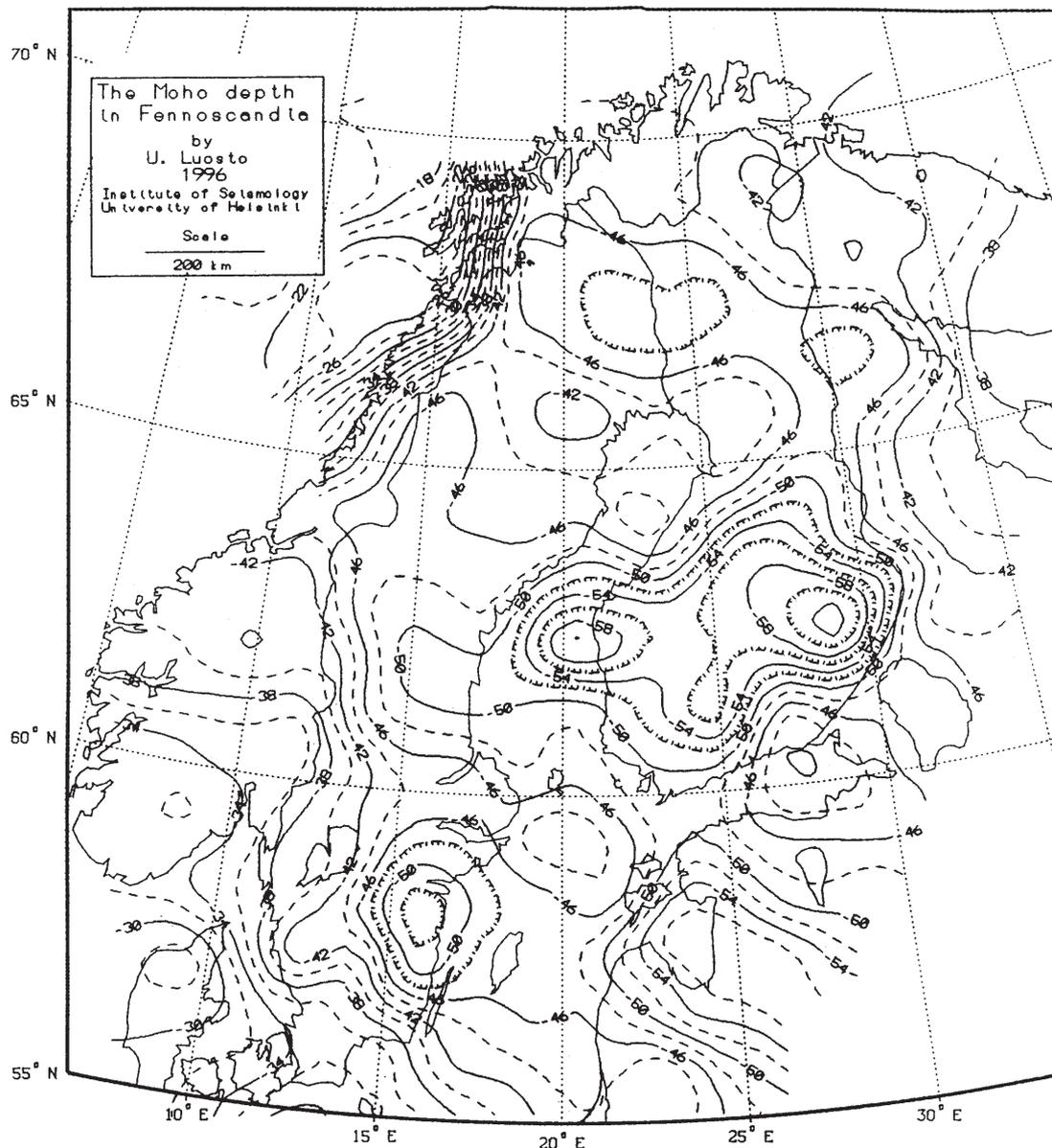
Fig. 4. Moho depth map calculated from the crustal thickness values of the profiles shown in Figure 1. Depths are given in km as negative values from the Earth's surface. The contour interval is 2 km. Pins in closing contour lines gives the direction of increasing Moho depth.
