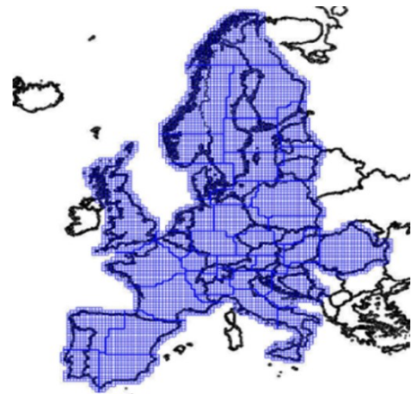
Fig. 3. NFEM meshes (thin blue lines) and “patches” (thick blue lines) for the computation of West European quasi-geoid by DFHRS (Jäger, 2018).
