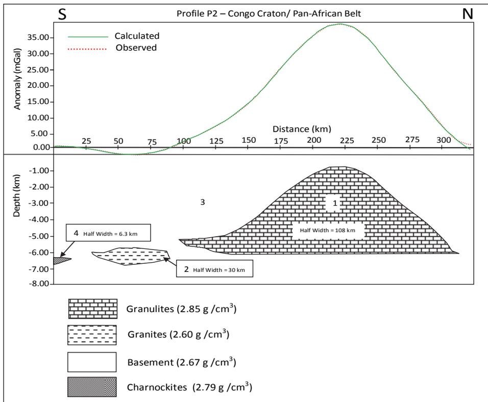
Fig. 7. Crustal model of profile P2.
