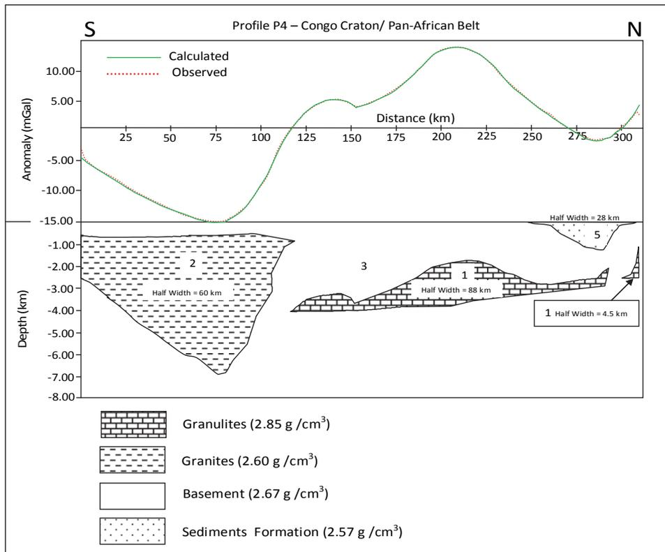
Fig. 9. Crustal model of profile P4.
