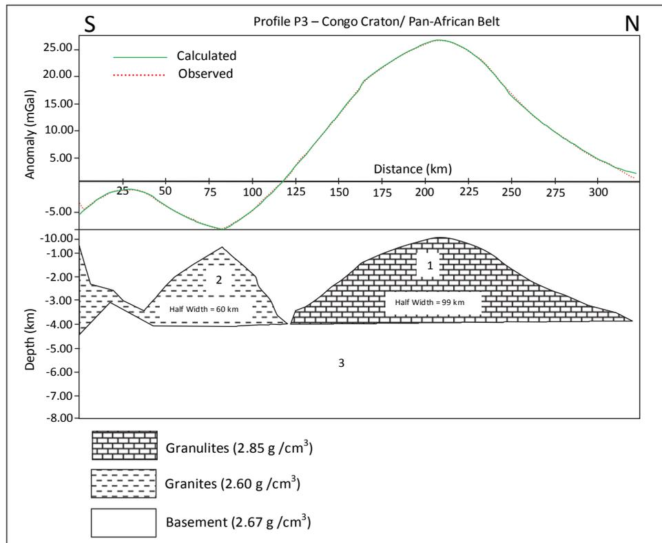
Fig. 8. Crustal model of profile P3.
