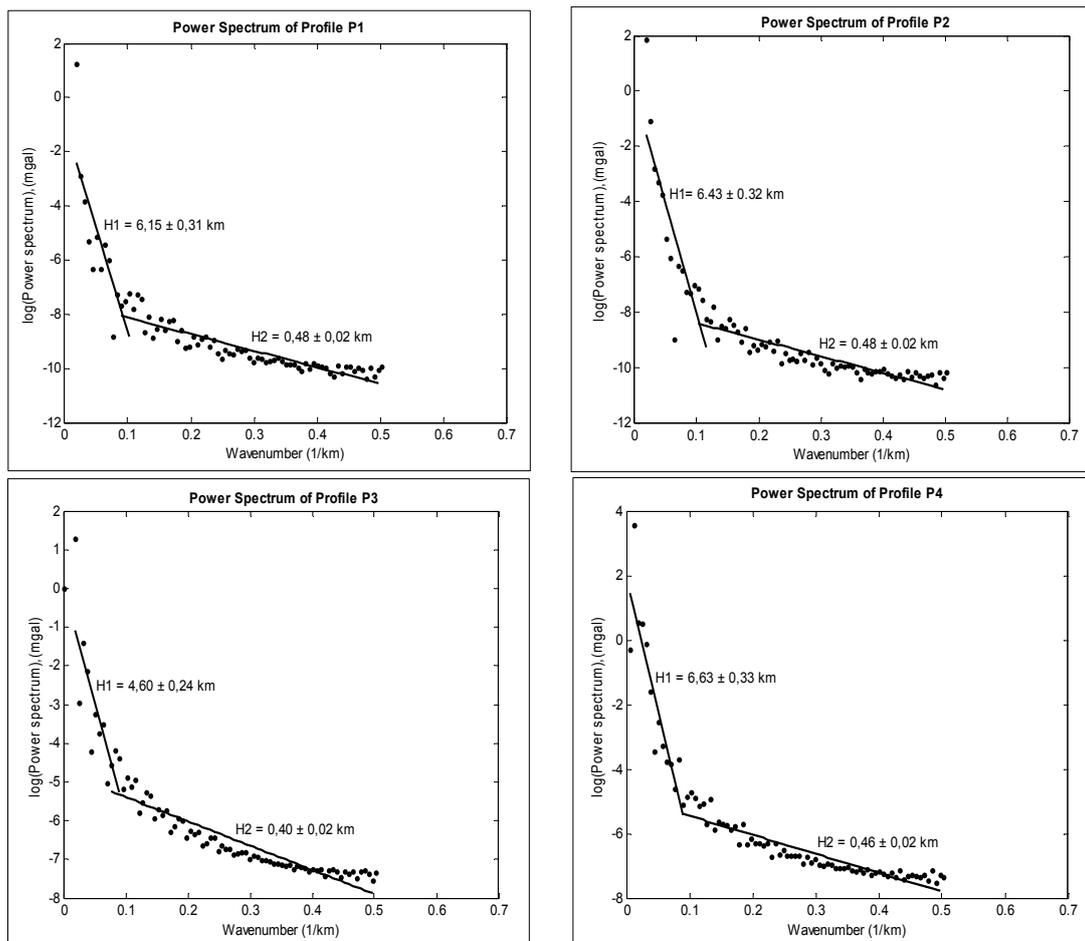
Fig. 5. Spectral analysis of profiles P1, P2, P3 & P4.
