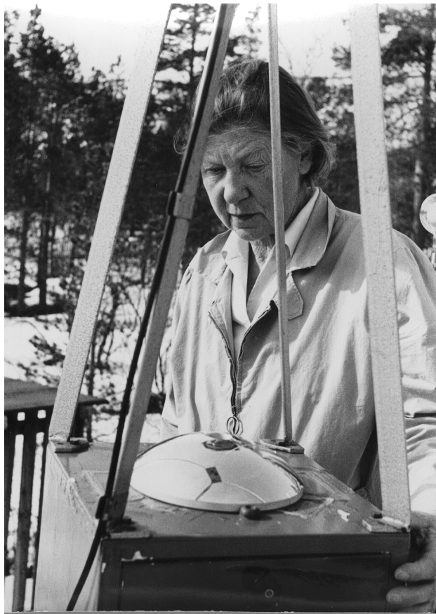
Fig. 13. Elsa Käck (1904–1984) at the Kevo station taking care of the second generation all-sky-camera with digital time and light standards produced with LED's. Colour films were used. (Photo by C. Sucksdoff, FMI photoarchives.)
