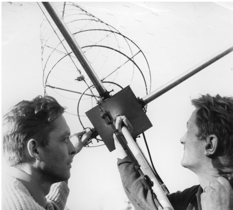
Fig. 10. Juhani Oksman (1931–) and Tarmo Mustonen (right) study a helix antenna for an auroral radar at the SGO in 1962. Later Oksman worked as professor and finally as rector at the UO. Mustonen specialised in servicing the ionospheric sounders and later the EISCAT equipment both in SGO and Lindau, Germany, and in Kiruna, Sweden. (Photograph by Tuulikki Mättö, Juhani Oksman's collection.)
