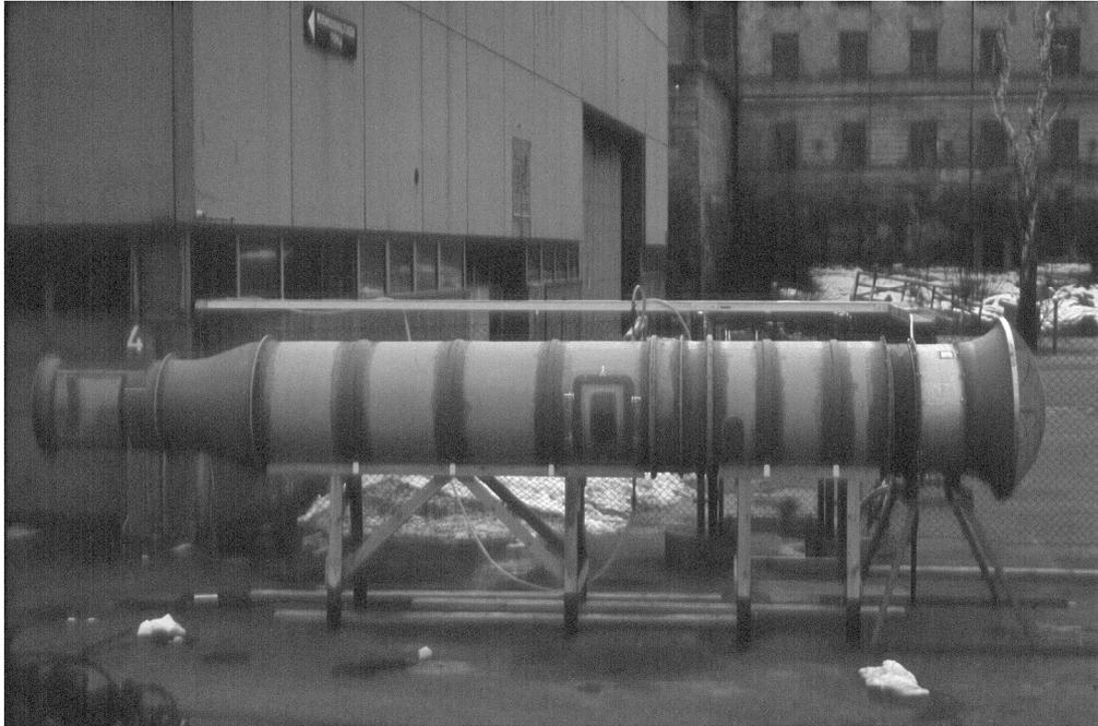
Fig. 7. Wind tunnel of FIMR for ice accretion experiments (courtesy of Lasse Makkonen).
