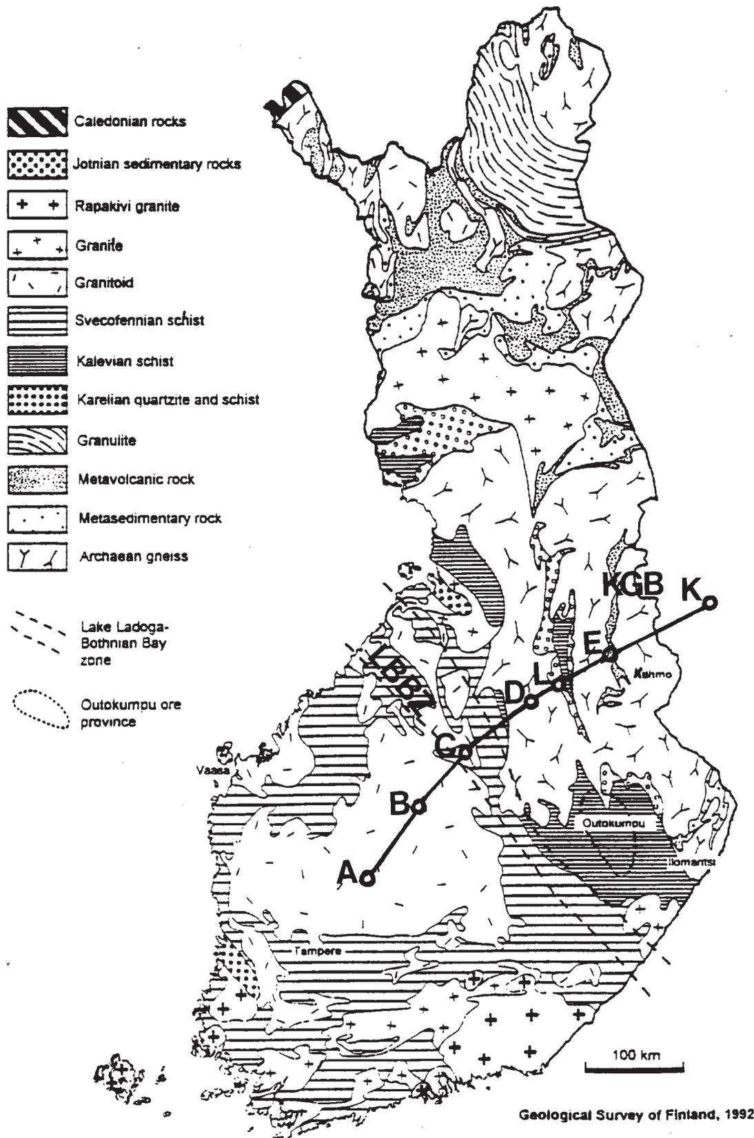
Fig. 1. Location of the extended SVEKA DSS refraction profile on the map of prequaternary rocks of Finland (after *Koljonen*, 1992). The capital letters A, B, C, D and E mark the shotpoints of the original SVEKA'81 profile. The letters K and L mark Kostamus (Russia) and Lahnaslampi (Finland) mining sites, respectively. LBBZ and KGB denote the Lake Ladoga-Bothnian Bay Zone and the Kuhmo Greenstone Belt, respectively.
