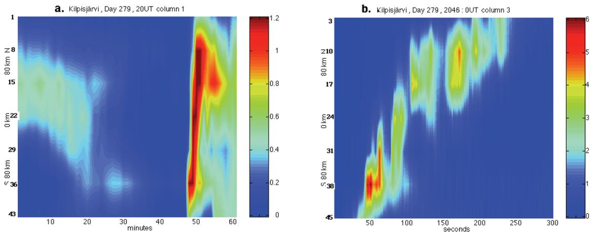
Fig. 3. a) Absorption images at Kilpisjärvi for column 1 (beams 1, 8, 15, 22, 29, 36 and 43) in north-south direction on 6 October 1994 in the interval 2000-2100 UT. The upper limit of the absorption scale is 1.2 dB. b). Absorption images at Kilpisjärvi for column 3 (beams 3, 10, 17, 24, 31, 38 and 45) in the north-south direction on 6 October 1994 in the interval 2046:00-2051:00 UT. The upper limit of the absorption scale is 6.0 dB.
