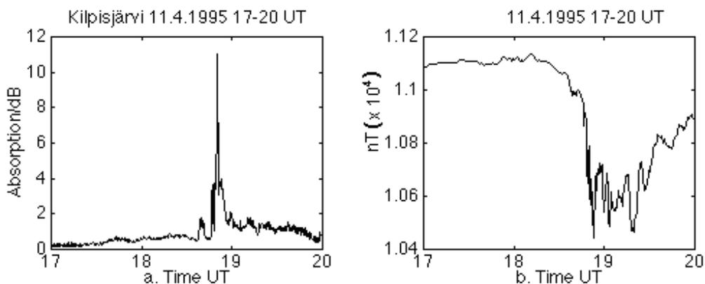
Fig. 7. a). Maximum absorption observed by imaging riometer at Kilpisjärvi on 11.4.1995, 17-20 UT. b) Magnetic X component at Kilpisjärvi on 11.4.1995, 17-20 UT.
