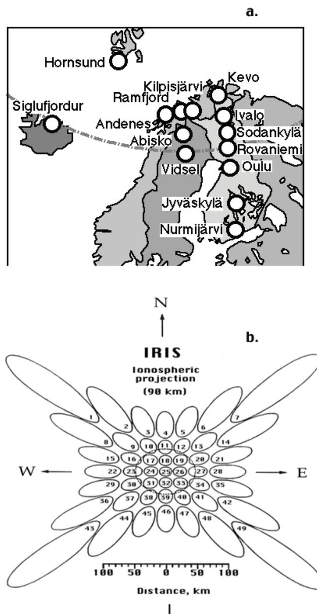
Fig. 1. a) Riometer stations. b). The patterns of antenna beams of the imaging riometer at Kilpisjärvi, at the height of 90 km.
