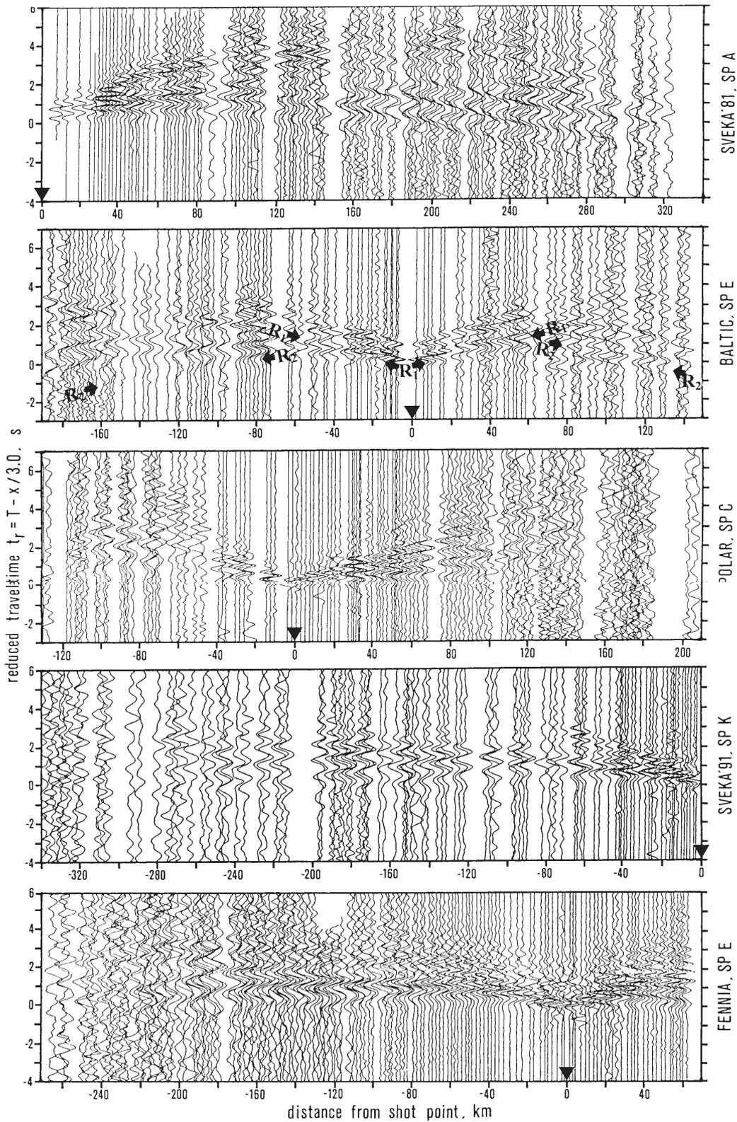
Fig. 2. Examples of amplitude normalized R-wave record sections for deep seismic sounding profiles SVEKA'81 (SP A), BALTIC (SP E), POLAR (SP C), SVEKA'91 (SP K) and FENNIA (SP E); vertical component; filter band 0.5-2.5 Hz; reduction velocity 3 km/s. Note two kinds of R-waves: "high" frequency waves R1 at distances up to about 50-70 km from the shot point and "low" frequency waves R2 at greater distances.
