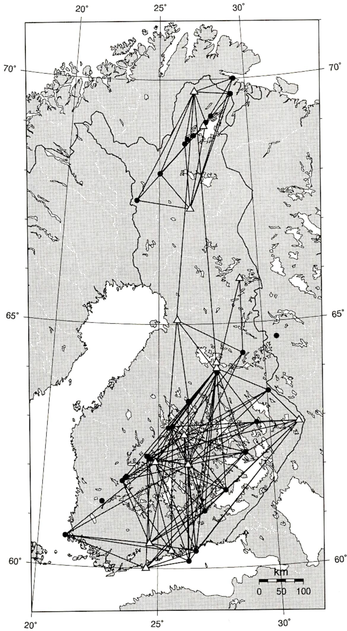
Fig. 3. Configuration of shot points and permanent seismograph station (marked by lines) for which amplitude - charge size dependencies were analyzed. Other explanations as in Fig. 1.
