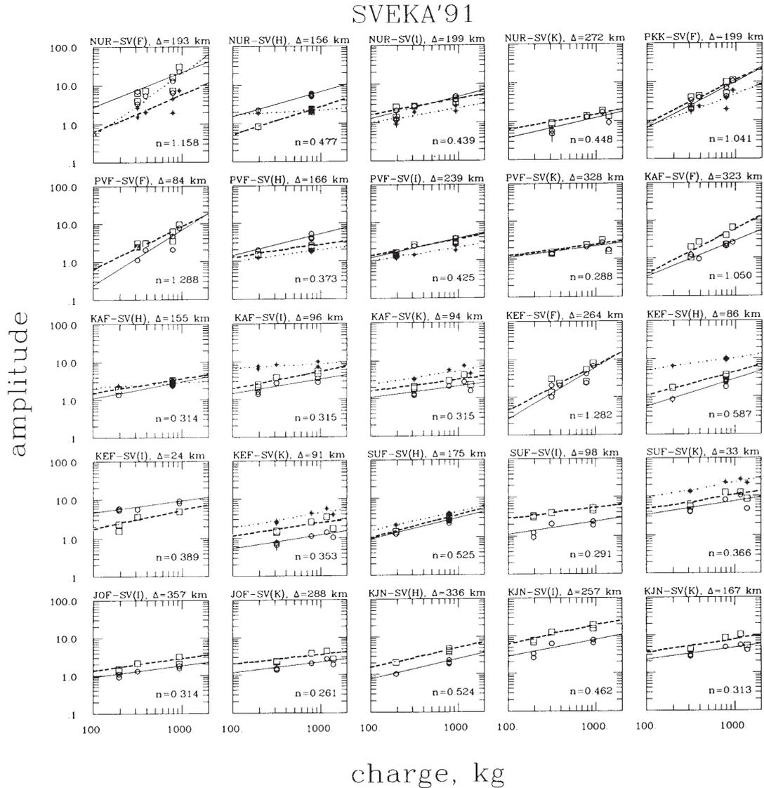
Fig. 6. Amplitude - charge size dependencies for the SVEKA'91 shots based on records at permanent seismograph stations NUR, PKK, PVF, KAF, KEF, SUF, JOF and KJN. The function (1) is fitted to the observed amplitudes; open circles and solid lines refer to P-waves, squares and dashed lines to S-waves, stars and dotted lines to R-waves); n = average value of exponent; Δ= distance from the station to shot point. Note the much bigger values of n for shot point F fired in the sea.
